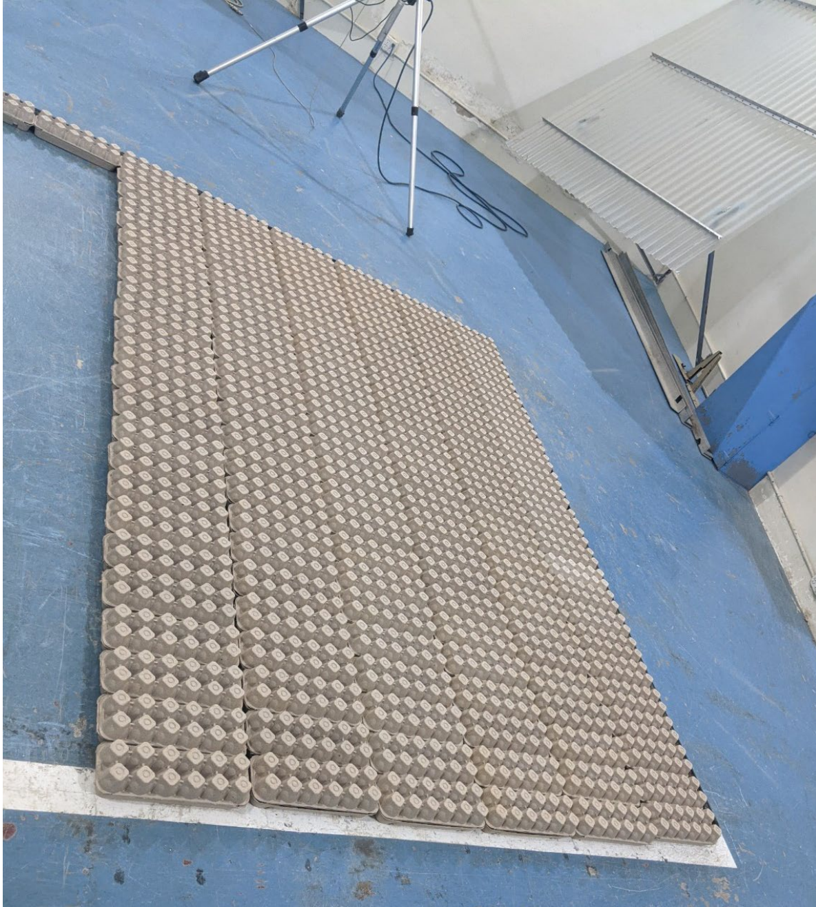
Figure 4 – Specimen egg cartons partially installed in test chamber
