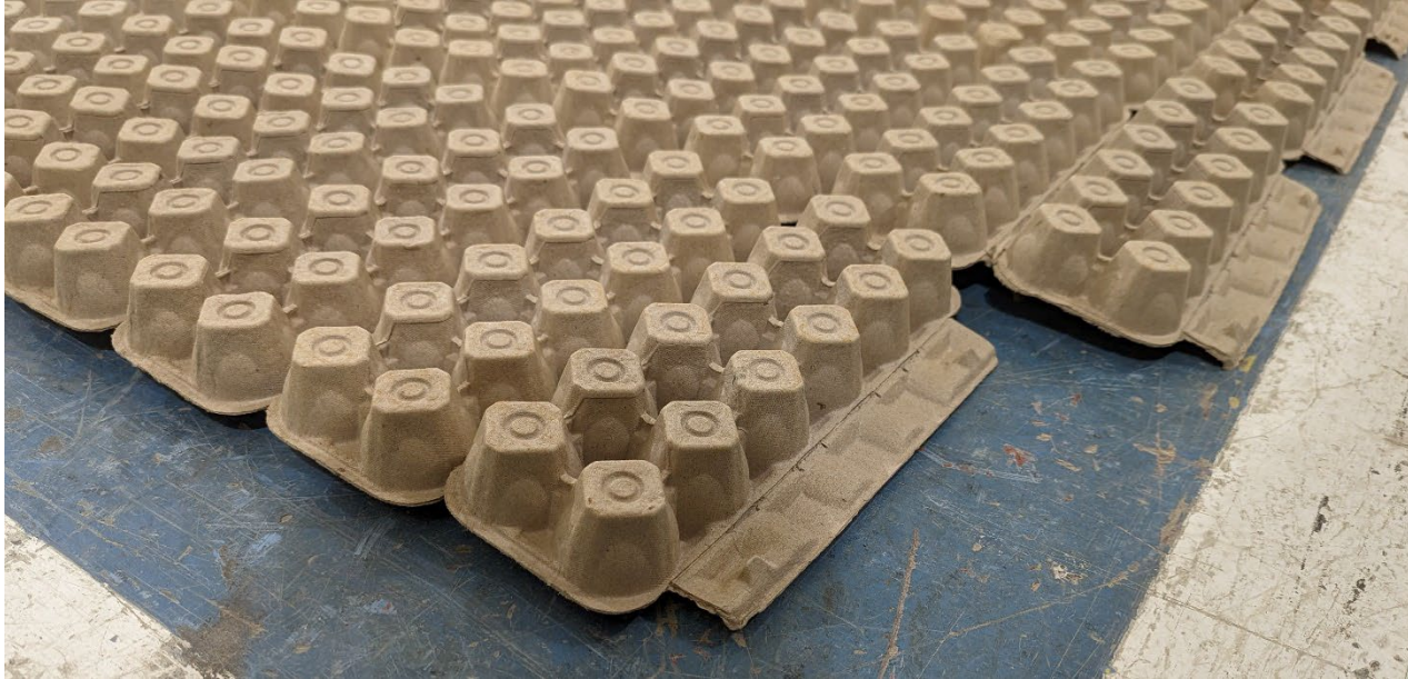
Figure 3 – Specimen partially installed in test chamber. Note that carton flaps are tucked under adjacent cartons.
