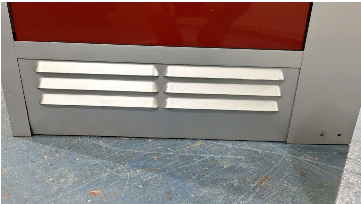
Figure 4 – Detail of vent openings at bottom of specimen
