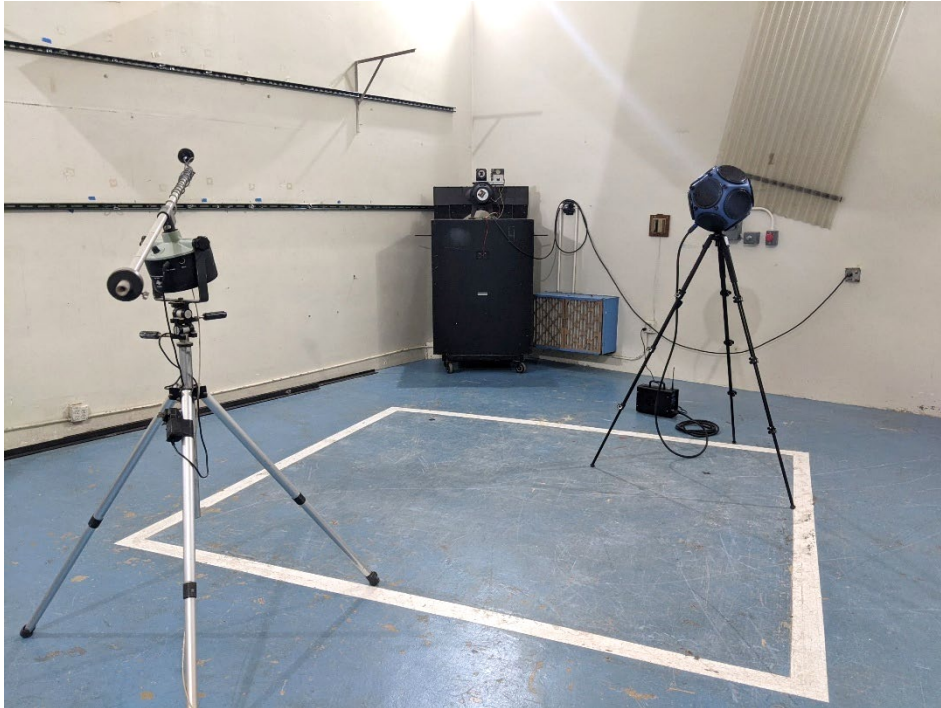
Figure 8 – Omnidirectional sound source installed after specimen removed from test chamber, position 1 of 2
