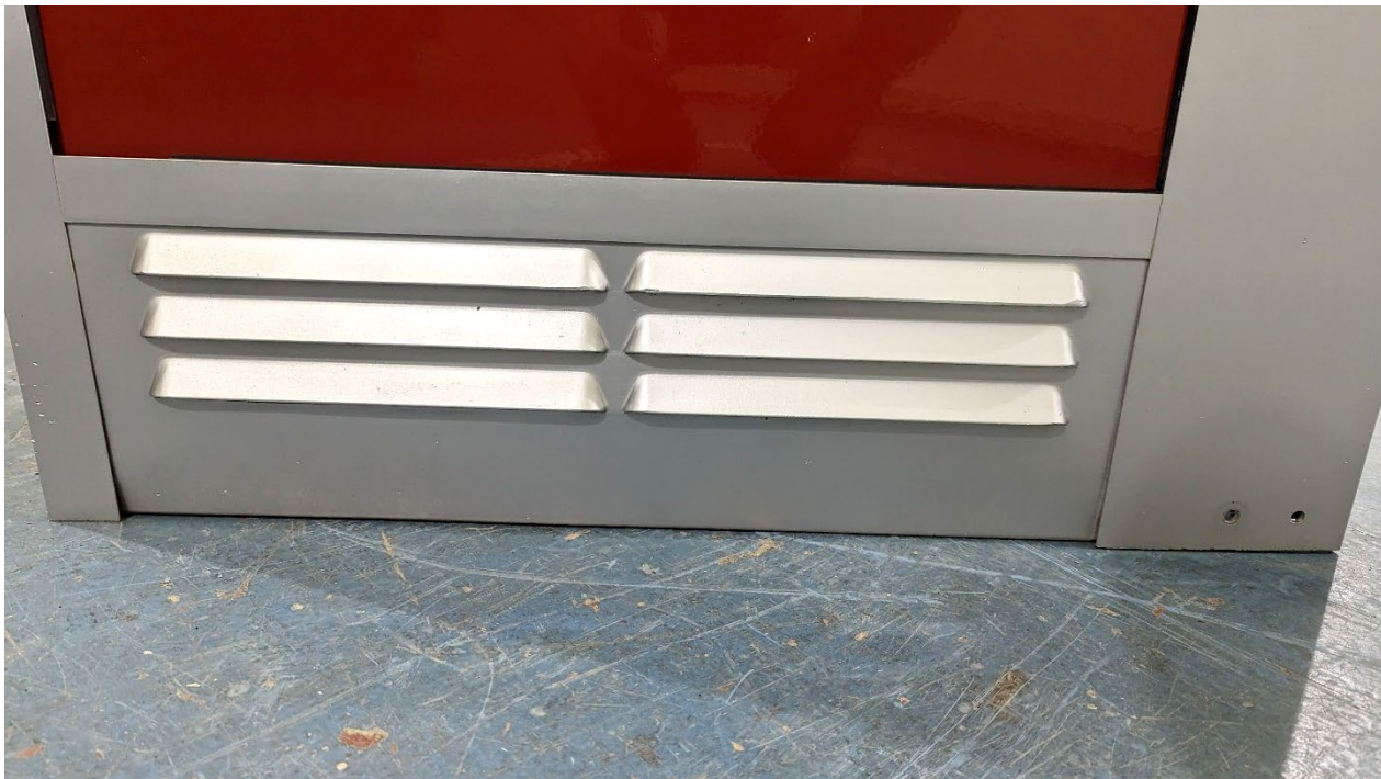
Figure 3 – Detail of vent openings at bottom of specimen
