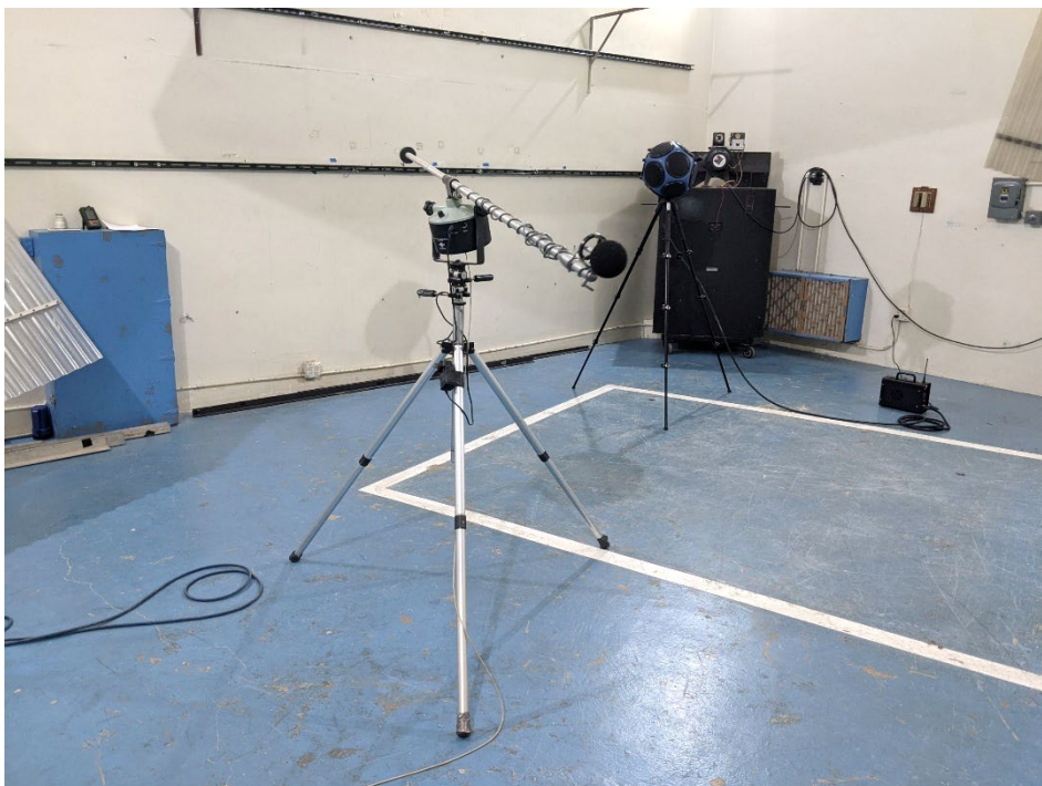
Figure 9 – Omnidirectional sound source installed after specimen removed from test chamber, position 2 of 2
